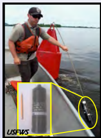
Kyle Mosel deploys a sonic receiver (inset) attached to a navigation buoy.
